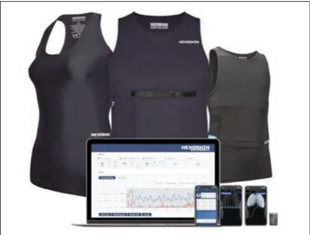
Fig. 3. Smart shirt with integrated ECG for heart monitoring, oximetry, respiration and temperature [4]
